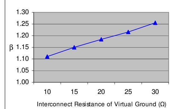
**Figure 3:  $\beta$ -variation on the growth of length (resistance) of the virtual ground interconnects**
