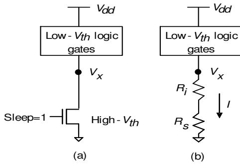
**Figure 1:** (a) Basic MTCMOS circuit structure, (b) The circuit model with sleep transistor and virtual ground interconnect modeled as resistors
