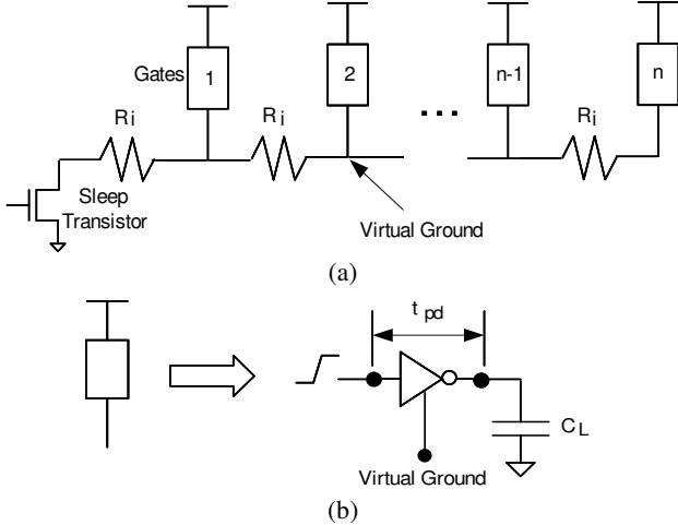
**Figure 2: (a) MTCMOS circuit structure, and (b) Simulation model for an inverter**
